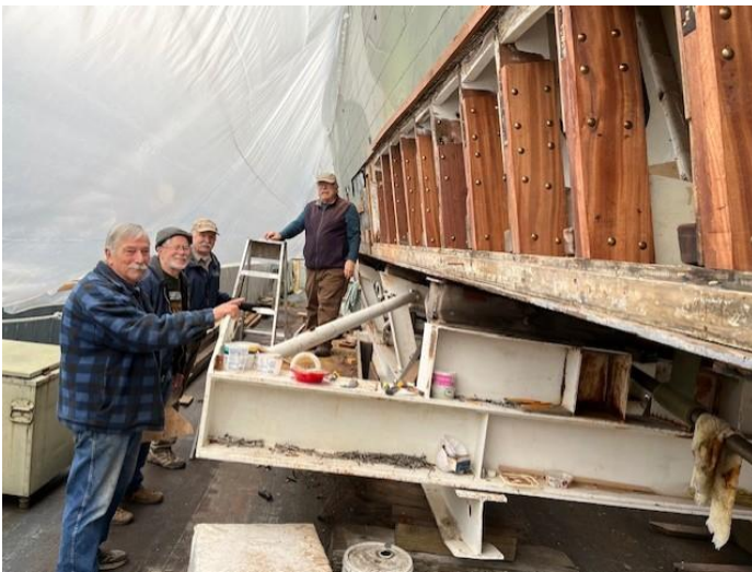
Tom Helping Replace PT Side Frames
