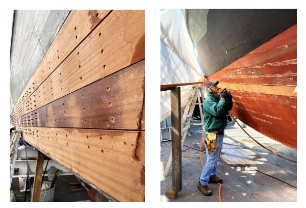
Some repairs to vertical frames in the bottom of the hull required removal of sections and replacement with new mahogany segments. Replaced segments are then bolted to the original frames with mahogany "sisters", shown in photo below left with Ron Taylor, Steve Stanage and Gary Veenker. Below right, Steve Stanage extracts himself from a tight space with limited access outboard of the engine room.
