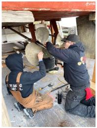
During the haul-out, we inspected/serviced the propellers and propeller shafts and replaced cathodic anodes (hull, rudder and propeller shafts). The center propeller was original size and larger than the port and starboard propellers, so we replaced it with the same size to match the other two to give us more consistent RPM, engine diagnostics and thrust. Our thanks to Sheffield Marine Propeller of Portland!
