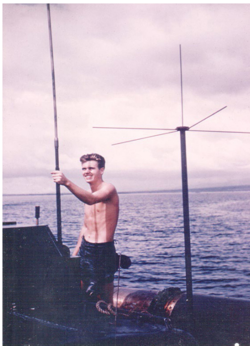
PT crewman extending the Premax radio antenna to its full 35 ft. height somewhere in the Pacific theater.
