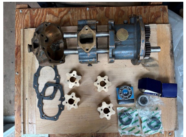
Seawater pump with new impellers, seals and bearings ready for assembly
