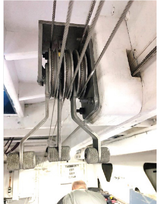
Engine room throttle as installed on PT 305
