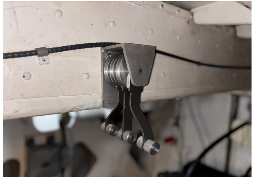
Newly Manufactured Throttle Control Levers positioned in PT 658 Engine Room
