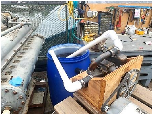
Left: Sea water pump installed on the Flow test fixture.
